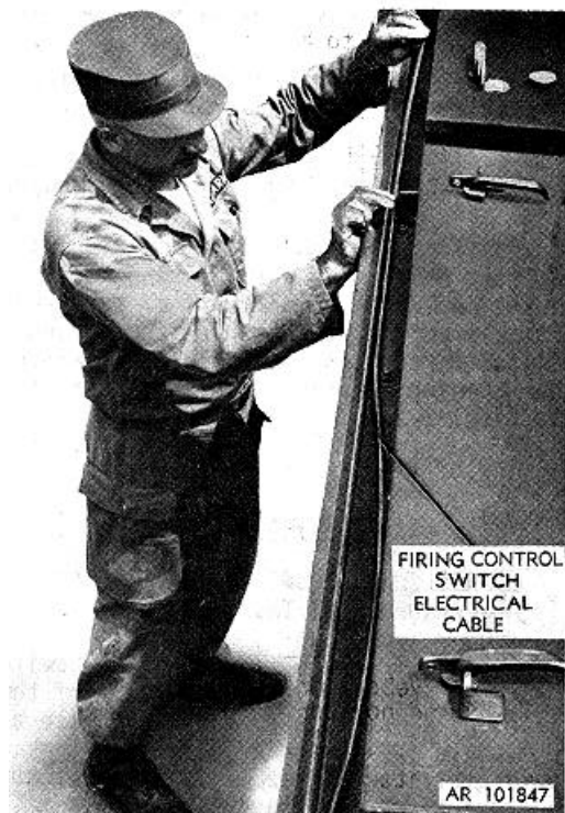
Figure 2-16. Placing firing control switch electrical cable along side of tow vehicle.
