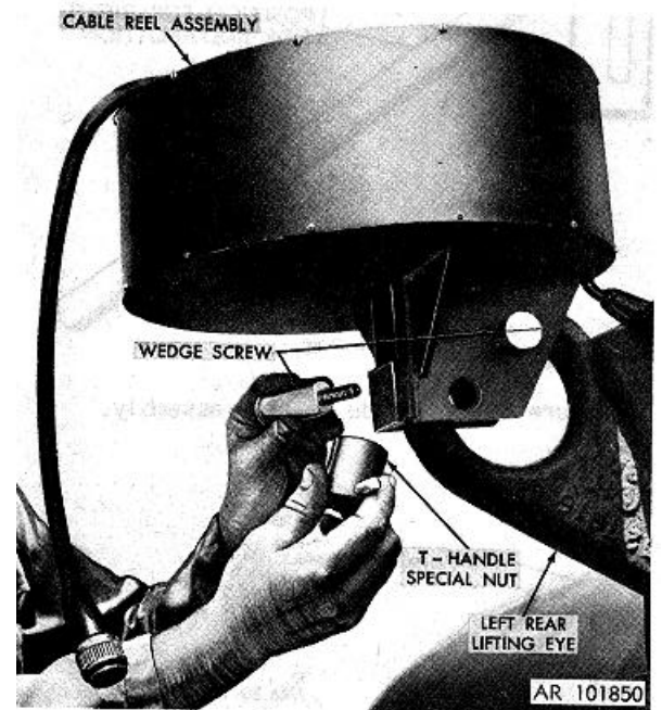
Figure 2-17. Securing cable reel assembly.
