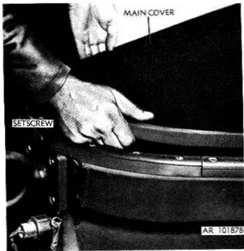
Figure 2-49. Lowering main cover into position.
