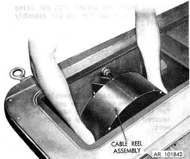
Figure 2-9. Removing cable reel assembly.
